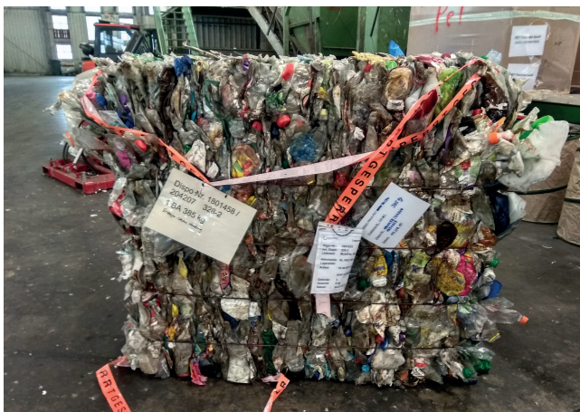
Bales of the specification mixed PET 70/30: during the material analysis the material was divided into the fractions other dimensionally stable PET packaging, trays with and without peeling film and blisters
