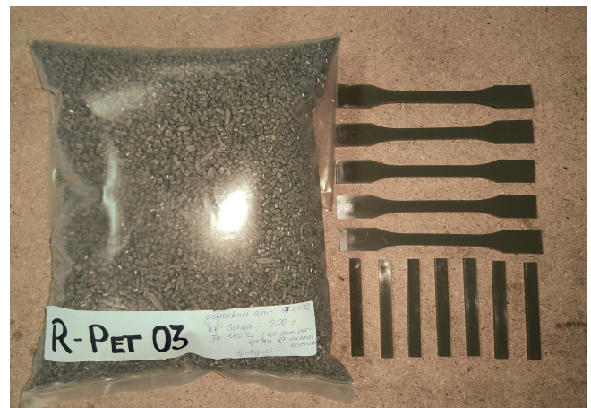
rPET blend compound and injected multi-purpose test rods
